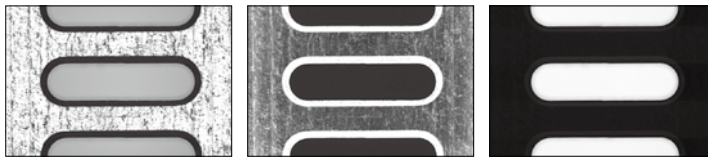
Vertical surface illumination Programmable ring light illumination Contour illumination
