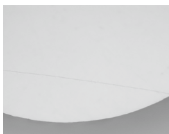
Scratched mirror-finished surface
