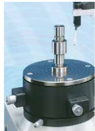
Automatic work piece alignment using servo-powered micrometers (AAT)
