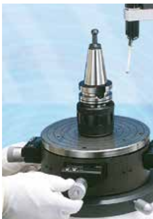
Digital micrometers for manual workpiece alignment (DAT)
