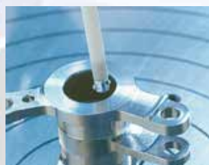
Roundness measurement, internal left: Flatness measurement
