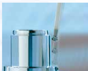
Cylindricity measurement across spiral line
