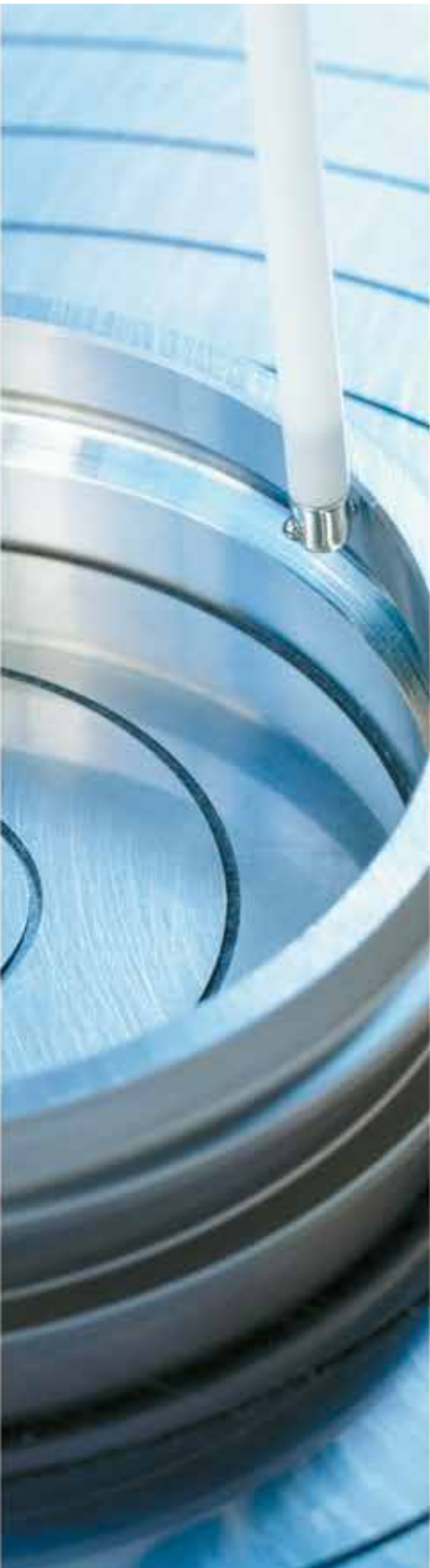
Cylindricity measurement across spiral line
