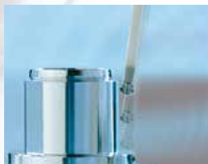
Cylindricity measurement across spiral line
