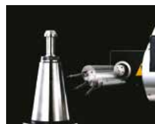
Probe system positionable in 1° increments
