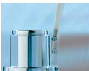
Cylindricity measurement across spiral line
